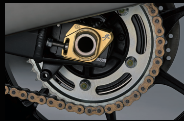
Aluminium chain adjuster 99117-10L00 Aluminium chain adjuster with Hayabusa logo. *Set of right and left side.
